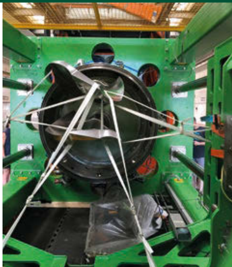
Professional securing of the machine during overland transportation by lorry.
