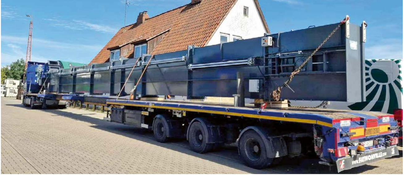
A sifting machine 8.70 x 3.70 x 3.90 metres, 23 tonnes
